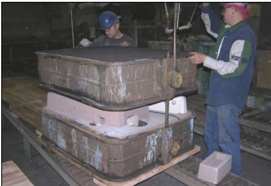
Finishing a KBB mold.
